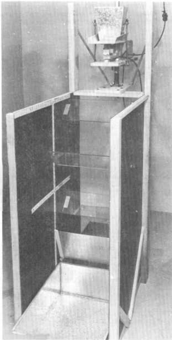
FIGURE 30.—Resilience separator with glass bounce plates.
