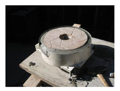
I cleaned up and left the mortar to dry for a couple days in the shade and then tried to reassemble the case. I discovered that the mortar at the outside edge was too high for the lip of the other case to fit in. I spent another hour carefully paring the mortar with a mason's chisel, attempting to fit the cases together, failing, and paring some more. The lesson, obviously, is to give plenty of room for the lip of the other case if you have a Meadows.
