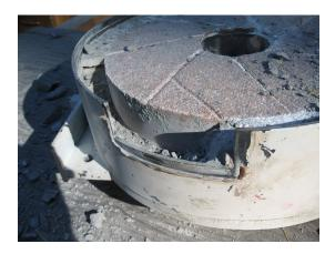
I found I had to be careful with the chisel to avoid damaging the edge of the case, which would make reassembly difficult. Once I got all the mortar out I used a big screwdriver to drive under the stone bit by bit, being careful not to crack the stone, until it popped loose. It still took some fiddling to get it off the grain cup.
