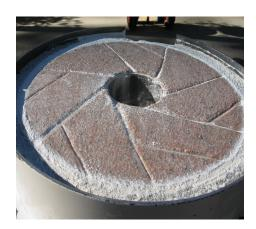
The first step in the process was to disassemble the mill. With the Meadows this only requires removing the hopper, feeder, and drive pulley and then the side of the case with the bed stone. The runner stone can remain in place because the stones will have to be "trained" to match after resetting the bed stone.
