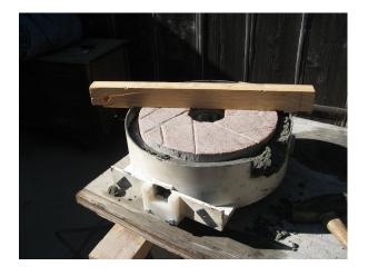
The last step was to fill in around the stone with mortar and taper it off away from the stone so milled flour can get to the case outlet. I quickly added the mortar and, using a narrow tile grouting trowel, got it pretty evenly shaped with a slope away from the stone to what looked like enough clearance for the edge of the other case that nests inside the bed stone case.
